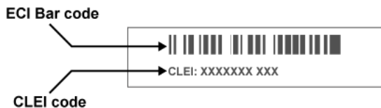
Figure 4: SFP+ bottom label
