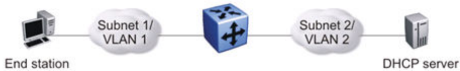
Figure 5: DHCP relay operation
