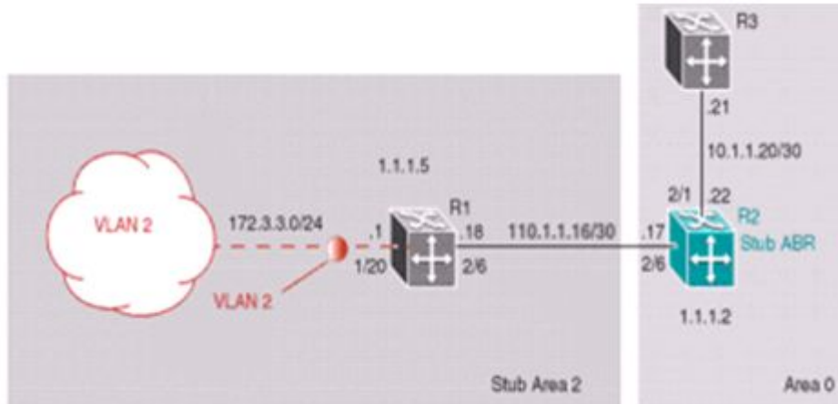
Figure 29: OSPF stub area example
