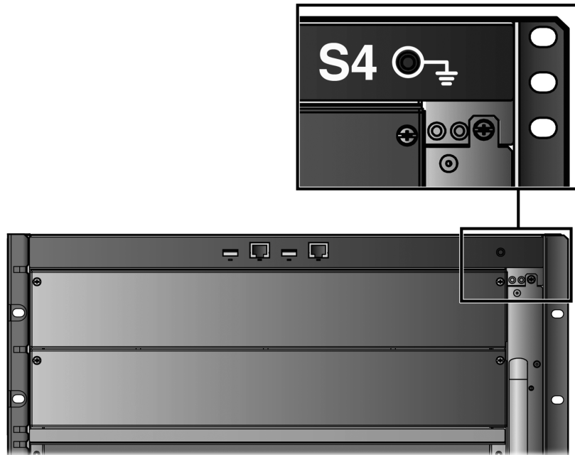
Figure 3-11 ESD Grounding Receptacle
