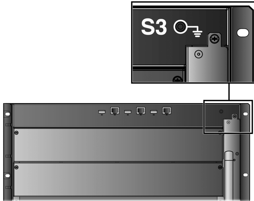
Figure 3-12 ESD Grounding Receptacle
