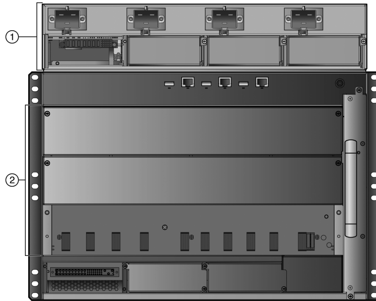
Figure 1-1 S3 Chassis with S-POE-4BAY-PWR PoE Subsystem
