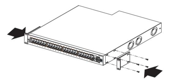
3. Slide the switch into the rack as illustrated.
