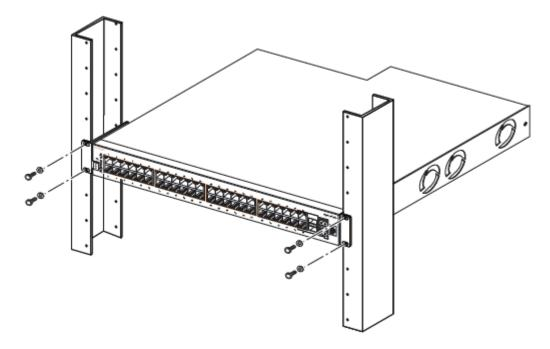
4. Insert and tighten the rack-mount screws.
