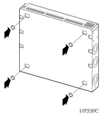
3. Set the switch on a table or shelf as illustrated below. Allow at least 2 inches (5.1 centimeters) on each side for proper ventilation and at least 5 inches (12.7 centimeters) at the back for power cord clearance.
