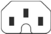
**Figure 4: IEC 60320 C16 connector**
