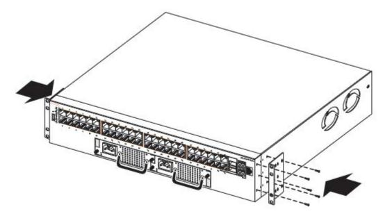
2. Slide the switch into the rack as illustrated.
