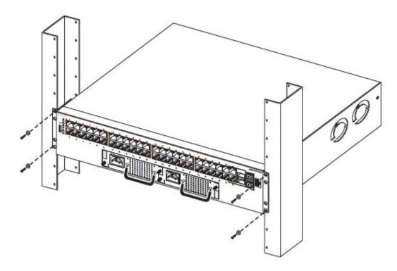
3. Insert and tighten the rack-mount screws.
