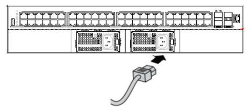
Figure 5: Connecting AC power to the front panel
