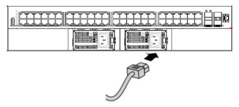
Figure 6: Connecting AC power to the front panel
