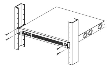
3. Insert and tighten the rack-mount screws.
