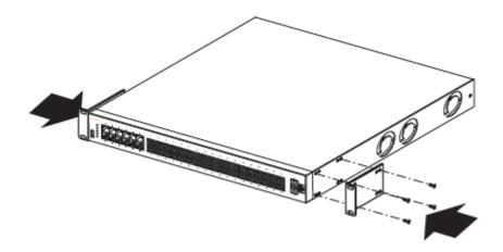
2. Slide the switch into the rack as illustrated.
