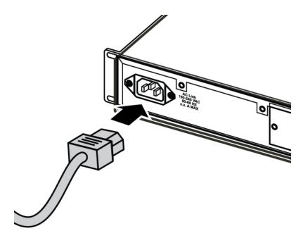
Figure 6: Connecting AC power to the rear panel
