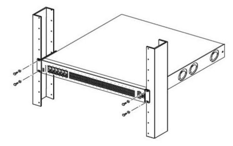
3. Insert and tighten the rack-mount screws.
