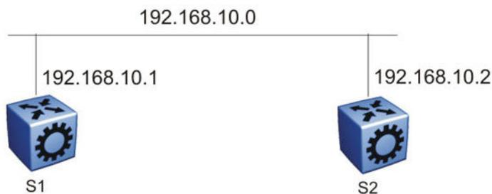
**Figure 15: Example 1: OSPF on one subnet in one area**
