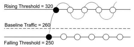
Figure 2: Alarm example, threshold less than 260
