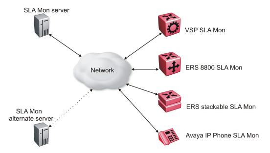
Figure 4: SLA Monitor network
