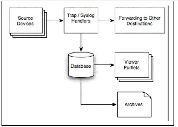
In terms of Traps/Syslogs Configuration options, the data flow proceeds as follows:
