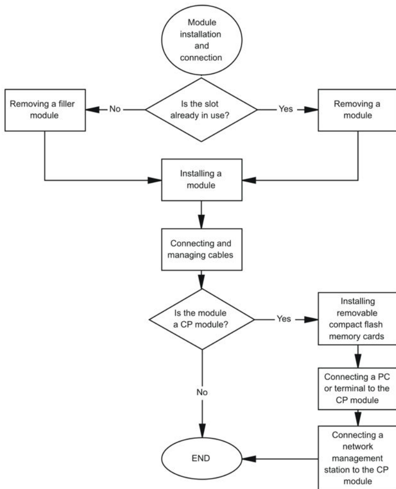
Figure 19: Module installation and connection procedures
