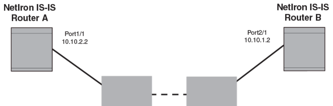
FIGURE 20 IS-IS Point-to-Point configuration
