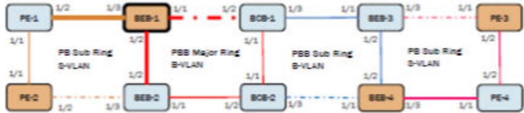
FIGURE 138 PBB interconnection node (BEB) sample configuration
