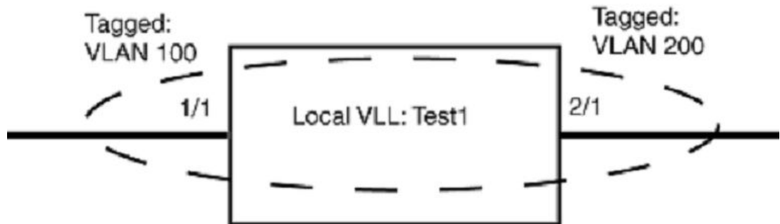
FIGURE 64 Local VLL "Test1" with two tagged VLANs
