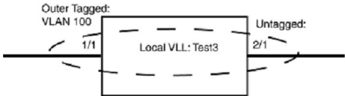
FIGURE 66 Local VLL "Test3" with one tagged VLAN and one untagged port
