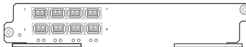
FIGURE 13 8x10GE-X module faceplate
