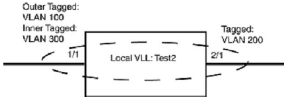
FIGURE 65 Local VLL "Test2" with one single-tagged VLAN and one dual-tagged VLAN
