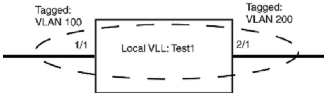
FIGURE 64 Local VLL "Test1" with two tagged VLANs
