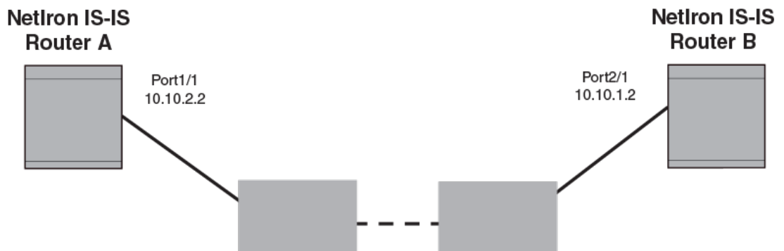
FIGURE 20 IS-IS Point-to-Point configuration
