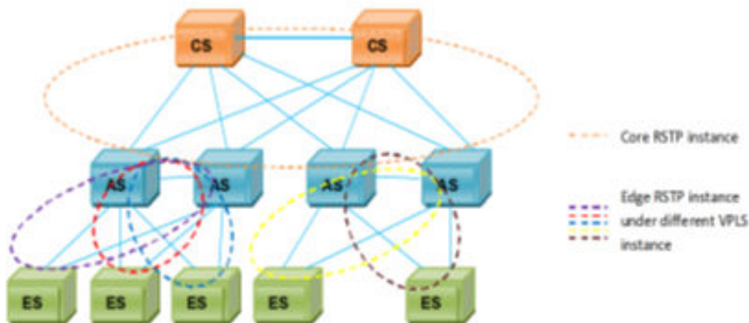
FIGURE 91 RSTP isolation in dual homing of AS and ES
