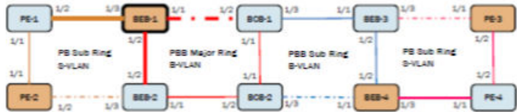
FIGURE 139 PBB interconnection node (BEB) sample configuration
