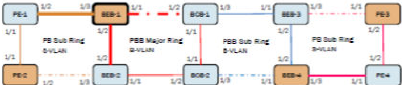
FIGURE 145 PBB interconnection node (BEB) sample configuration
