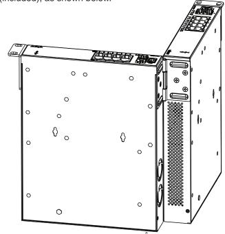
3. Attach the standard rack mount bracket ears to the outer end of each switch as shown below.
