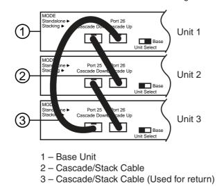
Base Unit Select switches To create a stack connection, order the appropriate Avaya Ethernet Routing Switch 3500 Series cascade cables to ensure fail-safe stacking. For stacking three or more units (maximum eight units per stack), order the 46 cm, 1.5 m, or 3 m cables as applicable (see "Before You Start" - step 3 for Order Codes).
