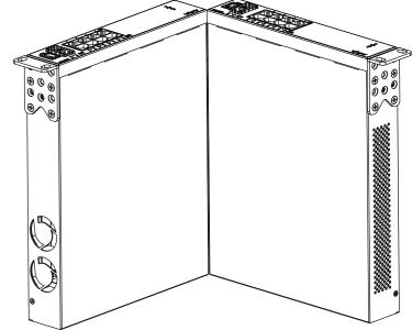
4. Once the switches are joined together, fold the hinged bracket inward.
