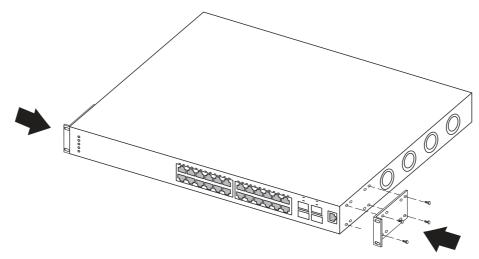
a. Slide the switch into the rack. Insert and tighten the rack-mount screws.
