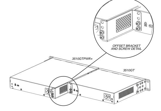
6. Slide the switches into the rack. Insert and tighten the rack mount screws.
