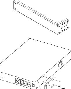
2. With the front of the ERS 3510GT or ERS 3510GT-PWR+ unit facing you, attach the long bracket from the optional kit to the left side of the switch using the flathead screws provided.
