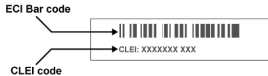
Figure 3: SFP+ bottom label
