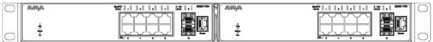
Figure 28: ERS 3510GT/3510GT-PWR+ Hinged mating bracket folded view
