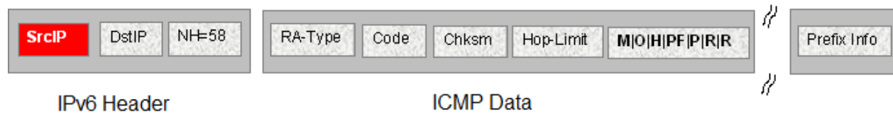
Figure 12: IPv6 ICMP RA data packet online
