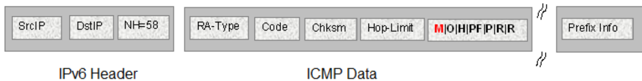
Figure 15: IPv6 ICMP RA data packet outline
