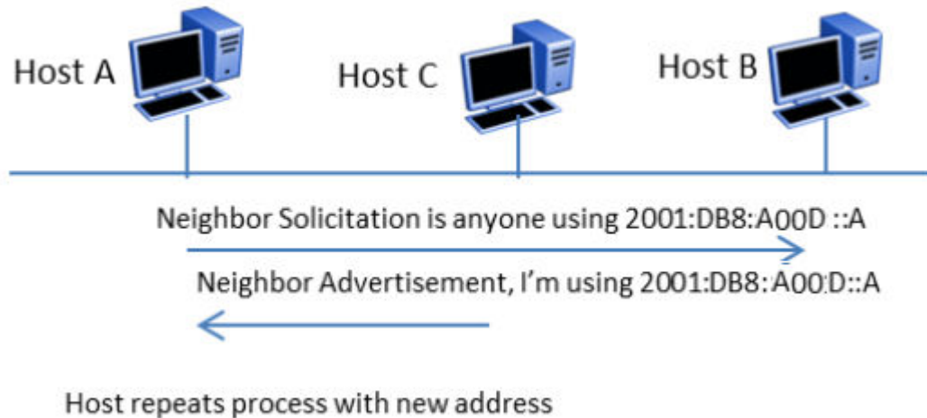
Figure 7: IPv6 Duplicate Address Detection
