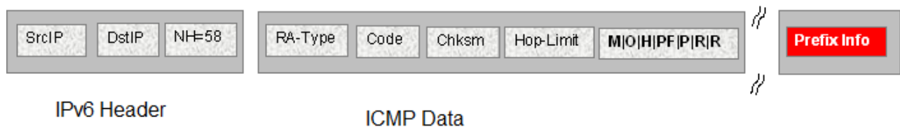
Figure 13: IPv6 ICMP RA data packet outline
