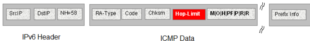
Figure 16: IPv6 ICMP RA data packet outline
