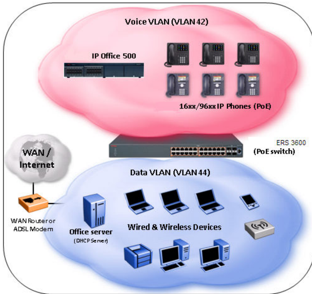
Figure 9: IP Office logical solution reference diagram
