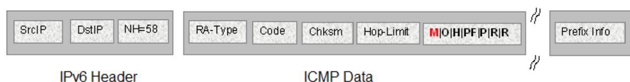
Figure 15: IPv6 ICMP RA data packet outline
