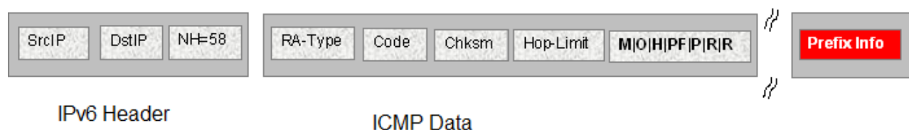
Figure 13: IPv6 ICMP RA data packet outline
