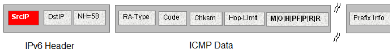
Figure 12: IPv6 ICMP RA data packet outline
