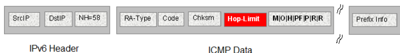
Figure 16: IPv6 ICMP RA data packet outline
