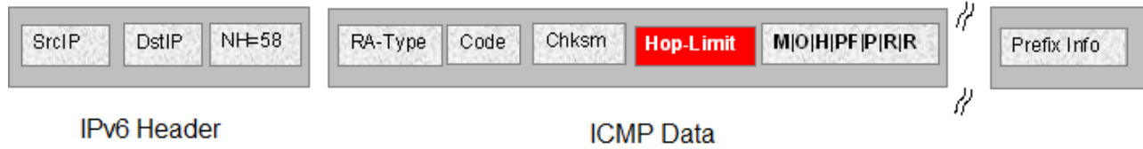
Figure 17: IPv6 ICMP RA data packet outline
