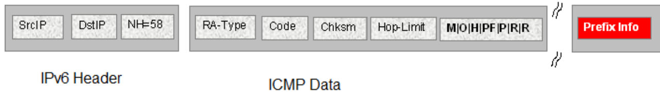
Figure 14: IPv6 ICMP RA data packet outline
