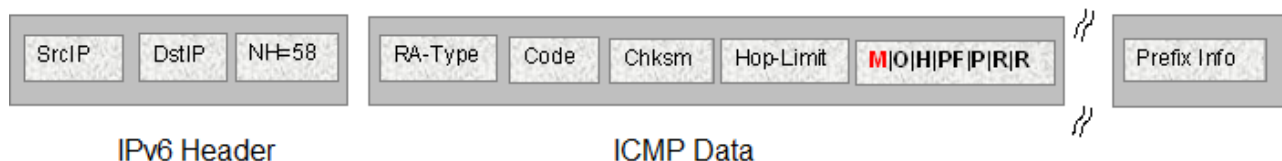
Figure 16: IPv6 ICMP RA data packet outline
