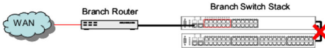
Figure 4: Remote Branch Office – Failure Scenario 3
