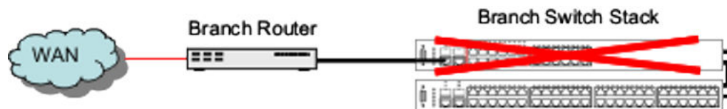
Figure 2: Remote Branch Office - Failure Scenario 1
