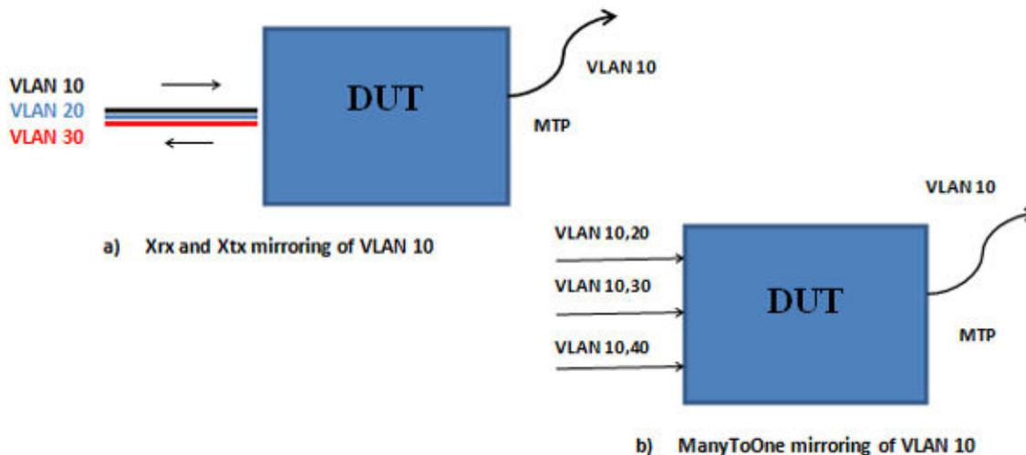
In the illustration, in example a, only the traffic from VLAN 10 (traffic received, sent, or both) is mirrored. In example b, there are multiple mirror ports, each of which is a member of several VLANs. This group of mirror ports is treated as a whole and only the traffic from VLAN 10 is copied on the sniffer port (MTP).
