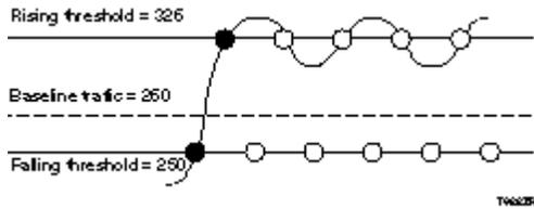
Figure 4: Alarm example - threshold less than 260
