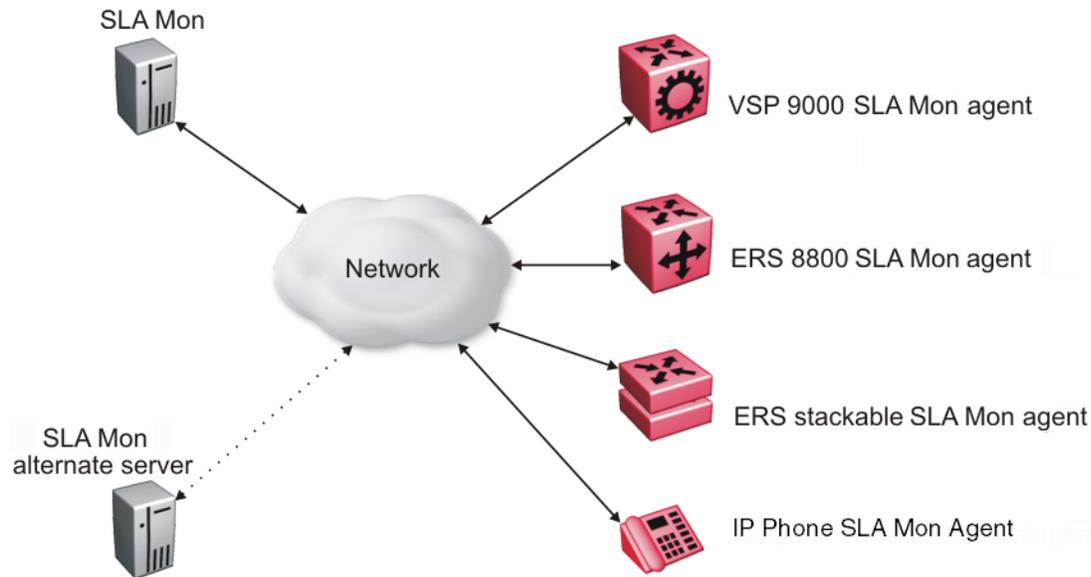
An SLA Monitor agent remains dormant until it receives a User Datagram Protocol (UDP) discovery packet from the server. The agent accepts the discovery packet to register with an SLA Monitor server. If the registration process fails, the agent remains dormant until it receives another discovery packet.
