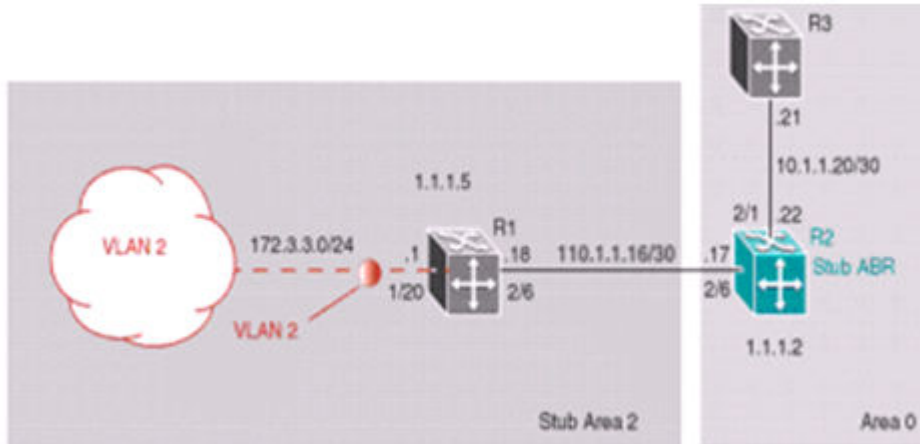
Figure 38: OSPF stub area example
