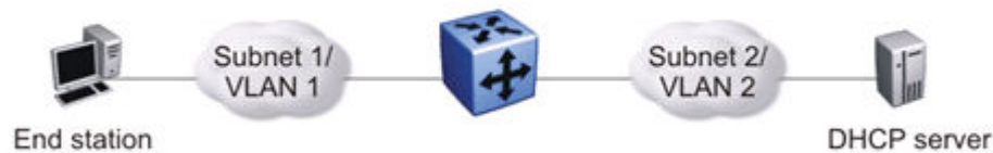
Figure 6: DHCP relay operation
