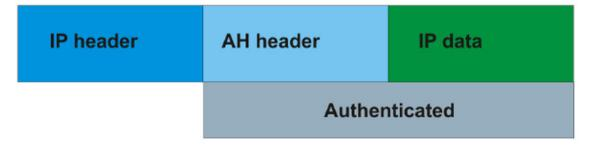
Figure 20: AH in transport mode
