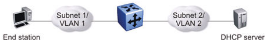
Figure 48: DHCP relay operation
