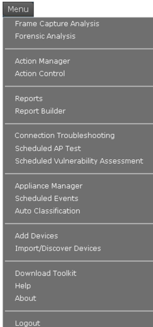
Most of the standalone features are Java applets. Reports and Help are web-based applications. Add Devices and Import/Discover Devices are an integral part of ADSP.
