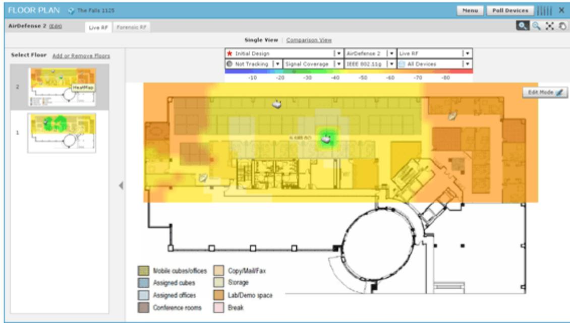
Live RF data is available on all Floor Plan pages. When the Floor Plan is refresh (manually or automatically), RF data is updated using the latest data (radio, power, channel, live status, etc.) about the devices. This data comes from the last polling cycle for the devices. If the **Poll Devices** button is clicked, the devices are refreshed first by ADSP and then the RF data is updated and displayed in the Floor Plan.
