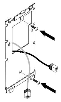
Mount the bracket to the wall so the Telco Box is ready available behind the mounting plate.
