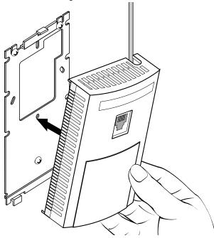
Once installed, connections are hidden from forward view, with only the physical infrastructure cables (Ethernet and power) extending from the AP-6511.
