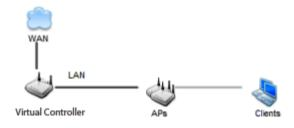
Bridge Mode - In Bridge Mode, the access point depends on an external router for routingLAN and VVAN traffic. Routing is generally used on one device, whereas bridging is typically used in a larger density network. Thus, select Bridge Mode when deploying this access point with numerous peer APs supporting clients on both the 2.4 and 5GHz radio bands.
