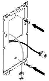
2. Connect one end of an RJ-45 cable into the wall mount connector on the AP-6511 as illustrated below.
