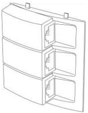
Remove the AP-6511's access cover by inserting a long pointed tool into the circular hole (opening) on the bottom of the AP-6511. Pull the access cover up and away from the AP-6511. Reverse the procedure to install the expansion module.
