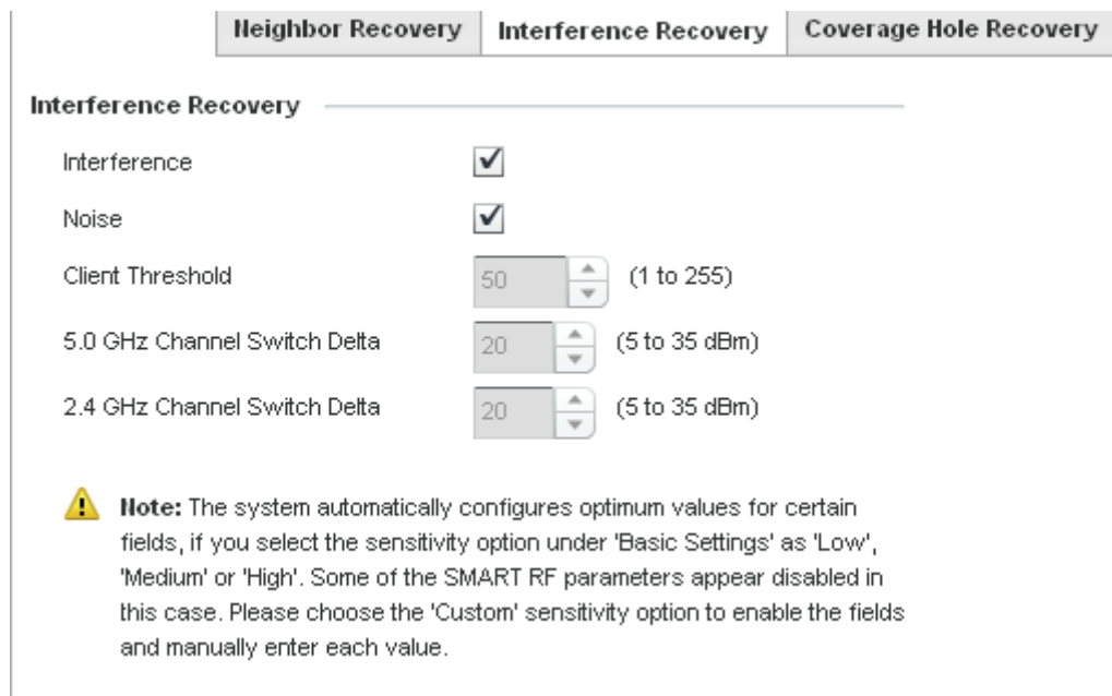
Figure 6-28 Smart RF Advanced Configuration screen - Interference Recovery tab
