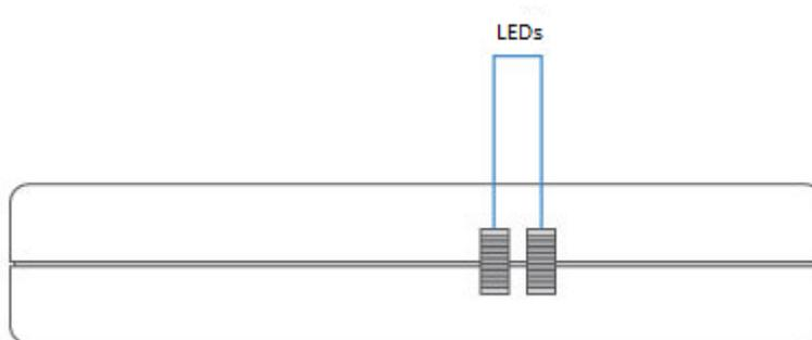
The LEDs provide a status display indicating error conditions, transmission, and network activity for the 5 GHz 802.11an (amber) radio or the 2.4 GHz 802.11bgn (green) radio.
