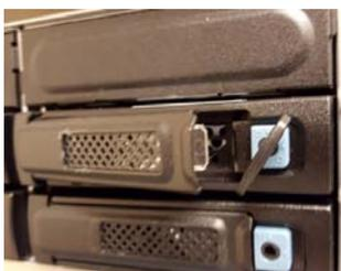
3. Carefully remove the HDD case from the NX-9600.
