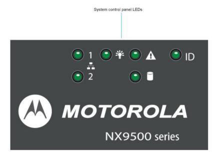
Remove the front bezel to access the control panel.
