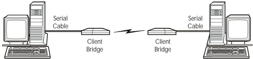
Two CB 1000s are required to perform wireless serial line replacement. Serial line replacement can operate with the radio in either Infrastructure or Peer-to-Peer mode. When performing Serial Line Replacement, data is exchanged using one of two protocols:
