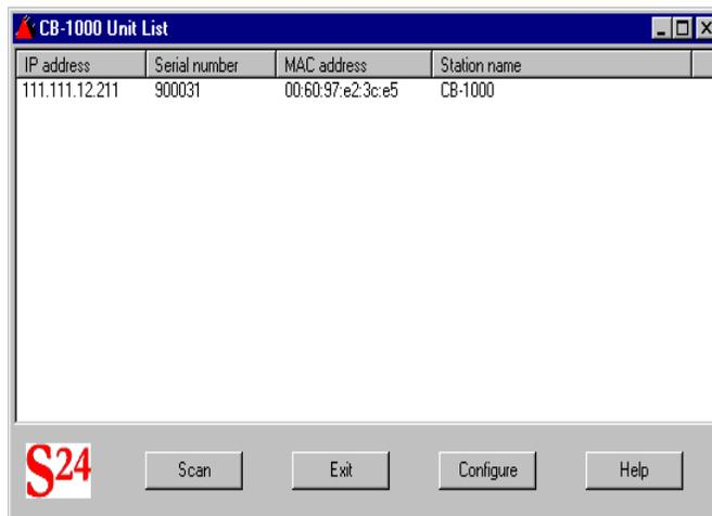
The *Unit List* window of the CB 1000 displays a list of CB 1000 units detected. All CB 1000 units can be controlled from this main window. The buttons on this window allow the user to SCAN, EXIT, CONFIGURE a unit, and display the HELP page. The SCAN function performs a search for active CB 1000 units. After a scan the display is updated with the available CB 1000 units.
