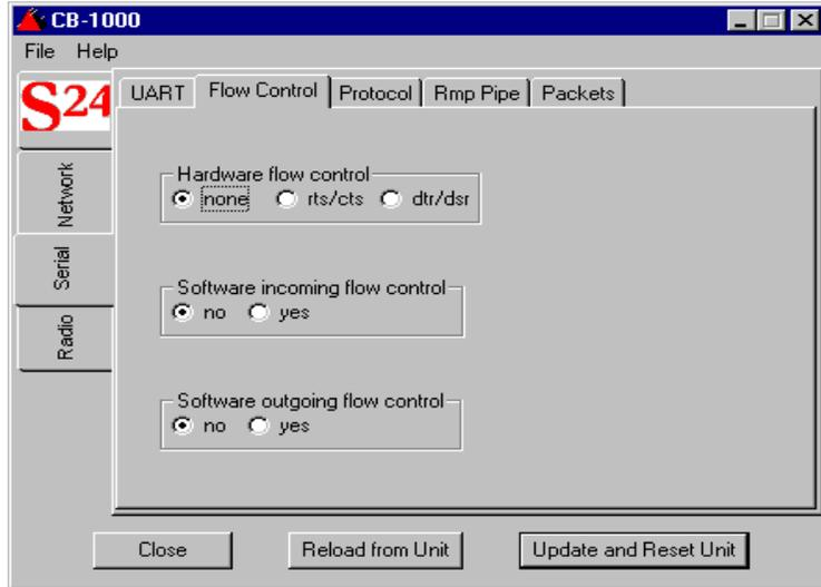
2. Check the flow control settings that match the device the CB 1000 is connected to.
