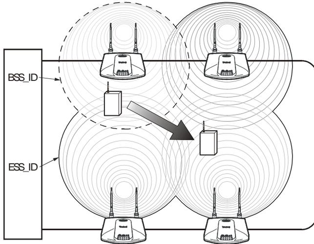
APs with the same ESSID define a coverage area. The MU searches for APs with a matching ESSID and synchronizes with an AP to establish communications. This allows MUs within the coverage area to move about or *roam*. As the MU roams from cell to cell, it switches APs. The switch occurs when the MU analyzes the reception quality and determines that a different AP can provide better service based on the best signal strength and lowest load distribution.
