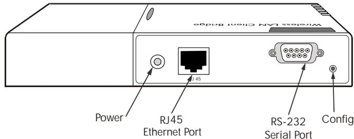
6. Plug the other end into the RJ-45 port on the CB 1000.
