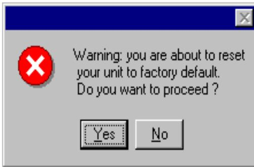
Depending on the current radio network setting, resetting to factory default could leave the CB 1000 unable to associate. Resetting to default resets all parameters, including the radio *ESSID*.
