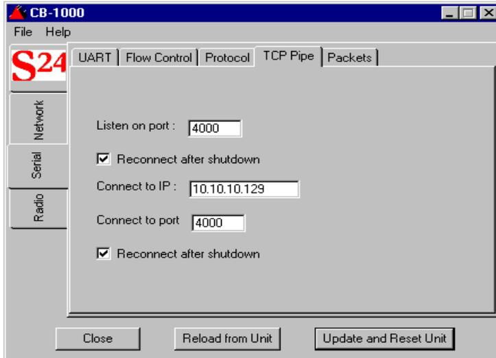
7. Set the Listen on port number for each unit to match the Connect to port number of the opposite unit. The defaults for both of these ports are 4000. Ensure a matching configuration by leaving the default values on both CB 1000s.
