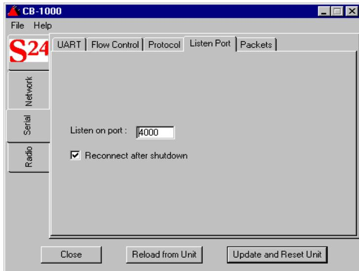
3. Type the port number the CB1000 listens for a connection. This is the port number the application uses to connect to the CB 1000. The default is 4000.
