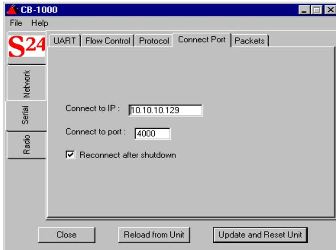
4. Enter the IP address of the device the CB 1000 is connecting to in the Connect to IP field.
