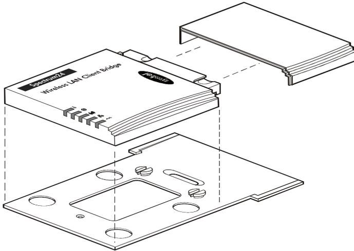
Remove the cap from the CB 1000 by pulling on the side of the cap to release it from the main CB 1000 assembly. Removal of the cap allows access to the radio card slot.
