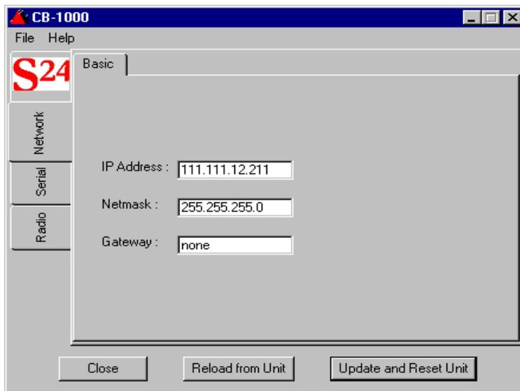
2. Enter an IP address assigned to the CB 1000. The IP address is the network address that other computers use to communicate with the CB 1000.
