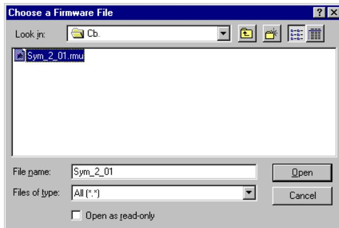
4. Double click on the file. The *Log Viewer* displays a progress status. At the end of the process, the CB 1000 resets. The *Log Viewer* indicates a successful update. The status light on the CB 1000 flashes, and after 15 to 20 seconds the new image is fully installed and the CB 1000 is ready for use.
