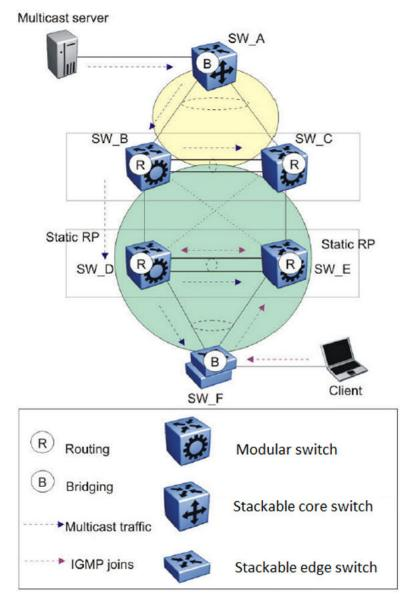
Figure 19: Multicast behavior in SMLT environment
