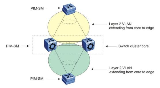
Figure 21: Multicast SMLT triangle
