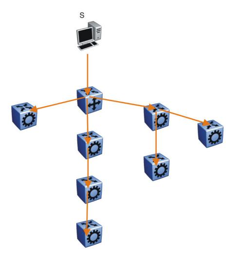
Figure 1: Multicast distribution tree and broadcasting
