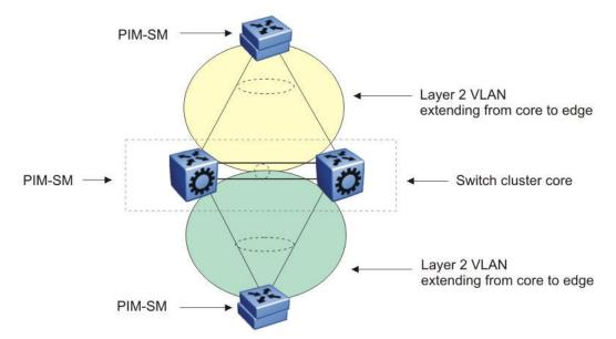
Figure 13: Multicast SMLT triangle
