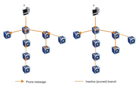
Figure 2: Pruning routers from a distribution tree
