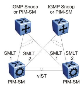
Figure 20: Multicast routing using PIM-SM
