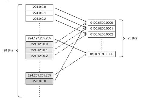
Figure 10: Multicast IP address to MAC address mapping
