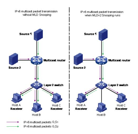
Figure 27: IPv6 multicast packet transmission when MLD v2 snooping is enabled and not enabled
