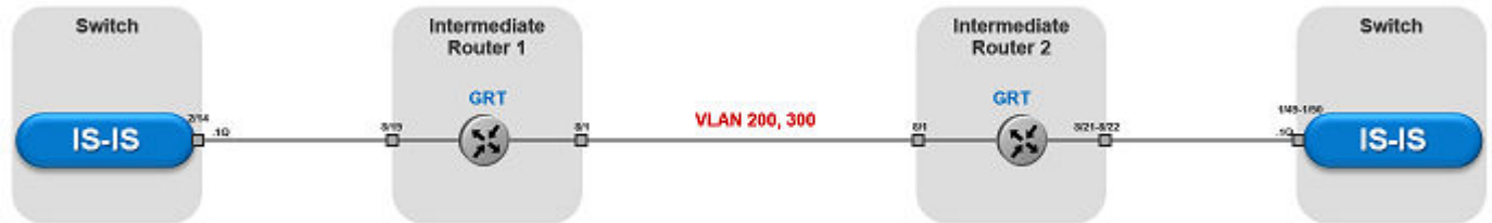
Figure 33: FE over Pseudowire traffic flow component view
