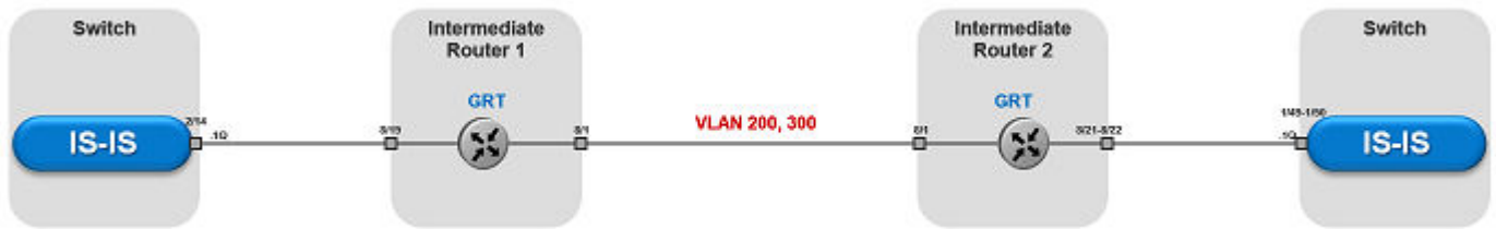
Figure 31: FE over Pseudowire traffic flow component view
