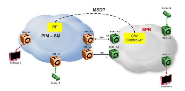
Figure 7: SPB-PIM Gateway base case configuration
