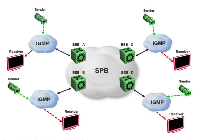
Figure 3: IP Multicast over Fabric Connect streams
