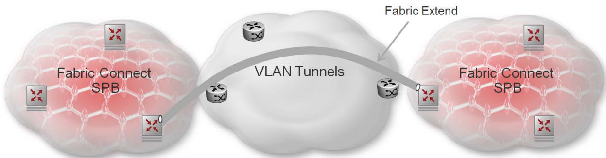
Figure 9: Fabric Extend over VLAN tunnels
